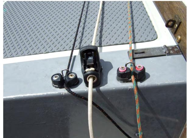
While I was about it I also ran the first reef point back to the cockpit (the white line). The tack cringle hooks over a hook made from a shackle with a lost pin. Incidentally I never bother with the lanyards for tying up the bunt of the reefed sail.
